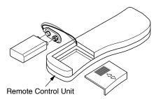
Figure 23 - Installing Battery in Hand-Held Remote Control Unit (CGHRCTB Series)
